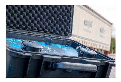
Using Jaltest PTE as power supply of the towed vehicle and without the need for a tractor head, you can connect to electronic control systems with the Jaltest diagnostic tool.
